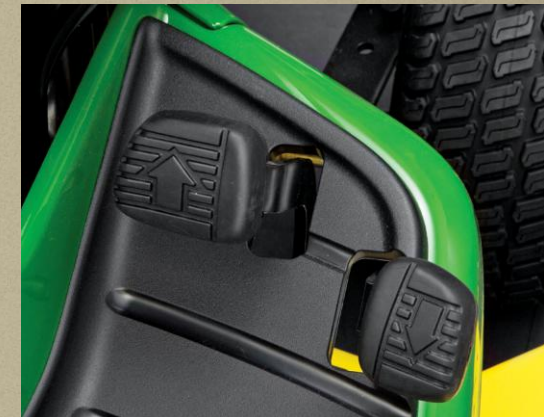
Twin Touch System. Twin Touch™ automatic transmission lets you easily change from forward to reverse with two-pedal foot control for effortless speed and direction changes. (Available on Select Series Tractors.)
